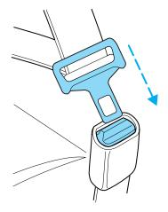
Grasp the shoulder portion and pull downward until the entire belt is pulled out.
